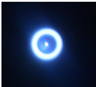
The fifth-generation Halo design operating during vacuum chamber testing
